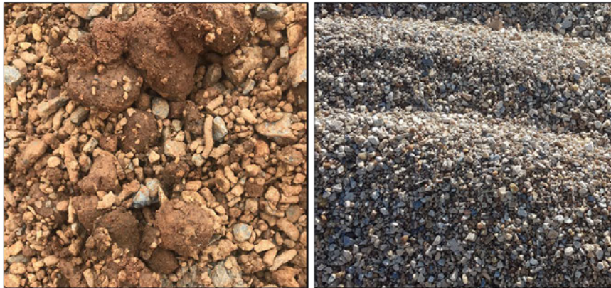
Figure 6. Gravel from Batches E to K. Gravel from Batch E (Left) after one round of treatment with clay balls and coating of fines. Gravel from Batches E-K after re-treatment (Right) showed removal of clay balls and the coating of fines.
