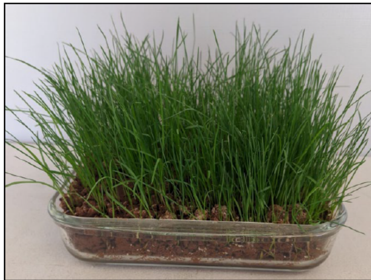
Figure 5. Extract of Treated and Reformed Batch V with 1% lime, soil pH 11 and approved RAAF Edinburgh grass mix successfully growing one month after germination.
