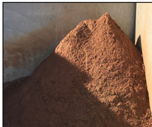
Figure 7. Sand in the material bay is red/brown in colour and homogenous.
